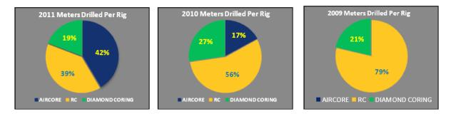
The meters drilled in 2011 were 42% Air Core, 39% RC and 19% Core as compared to 2010 were 17% Air Core, 56% RC and 27% Core. These proportions, however, vary from year to year. RC drilling is the method of choice for obtaining consistently high quality rock samples with speed and efficiency, while the pricing of RC drilling allows clients to extend their budgets.
